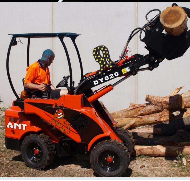
The Angry Ant 620 Mini Loader packs a powerful punch, plus the added manoeuvrability of front articulation and hydrostatic 4WD. Powerful enough to handle the heaviest of loads and compact enough to work in tight areas. Quality engineered and backed by an experienced Australian service and parts network, you can rest assured your Angry Ant will give you many years of loyal service. With all the attachments available, your Angry Ant is ready to tackle any task you can throw at it.
